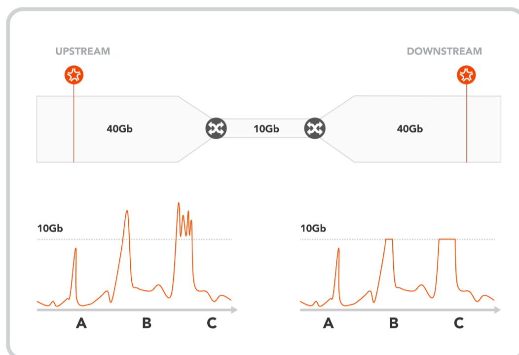
Figure 5. Microbursts measurements made at different points on the network
